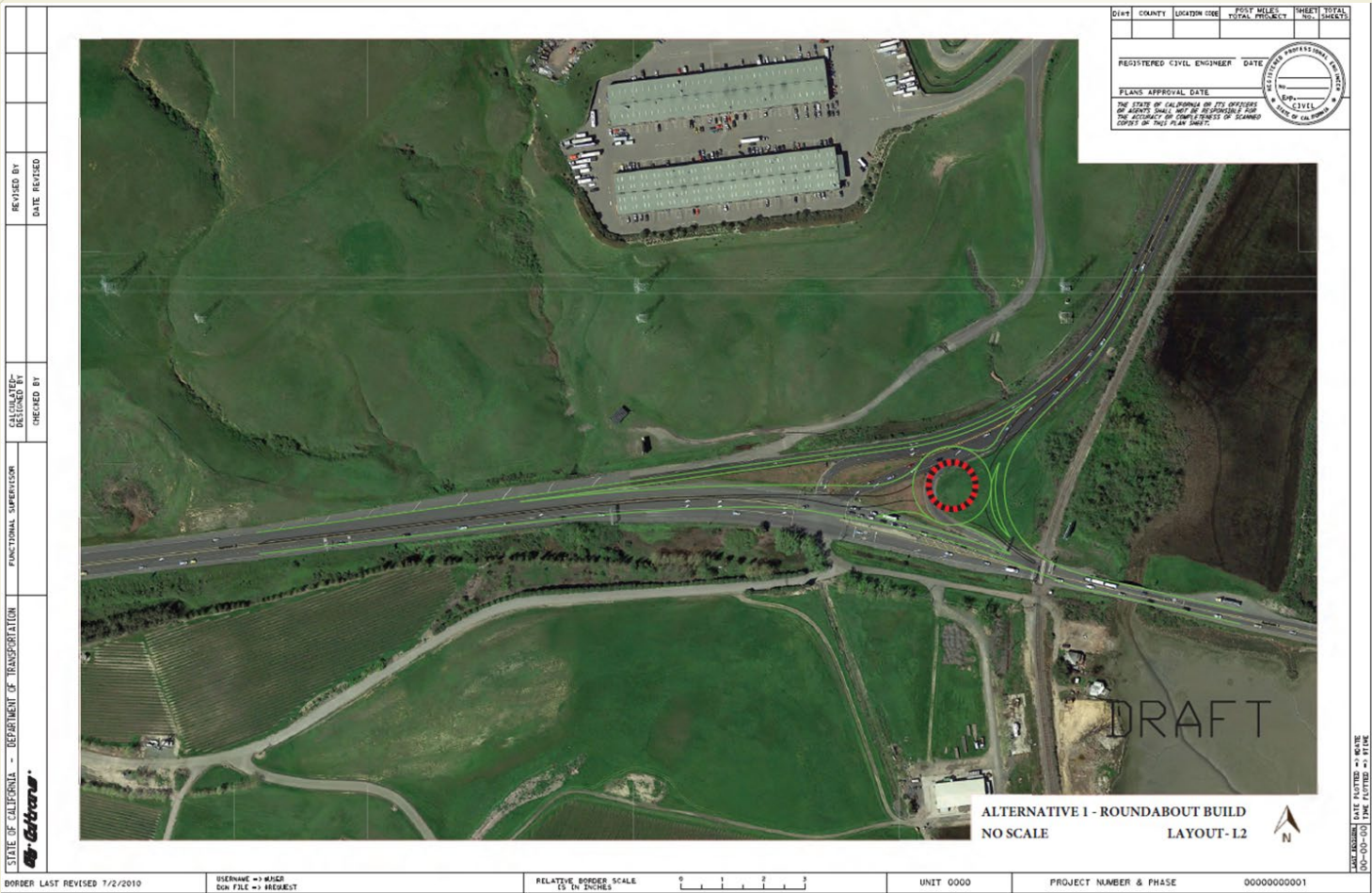
Build Alternative 2: (Auxiliary) Merge Lane Extension with Roundabout
