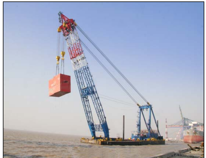
Testing of the Shearleg Crane Barge at ZPMC
