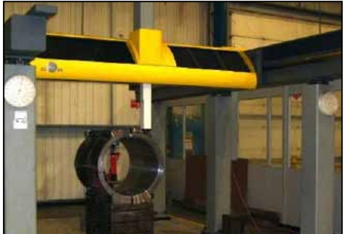
Cable Band Undergoing Dimensional Inspection
