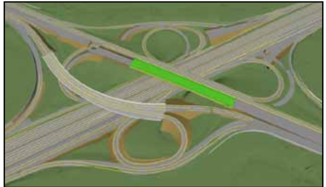
Stage 2 - Demolish and Replace South Side of Route 92 Separation Structure
