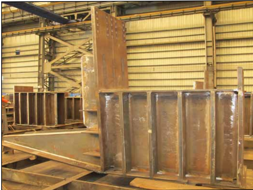
Roadway Box 12 Cable Brackett
