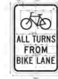
R (SPECIAL) "ALL TURNS FROM BIKE LANE" R0-23a (12"X18") SPECIAL BICYCLE SIGNS NTS
