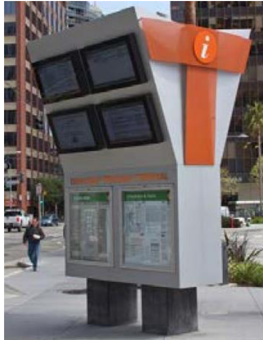
Sign type example from section 2.6 of MTC Guidelines: Real-time Information Display Systems
