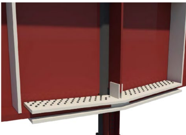
4. Bolted sandwich plate repair
