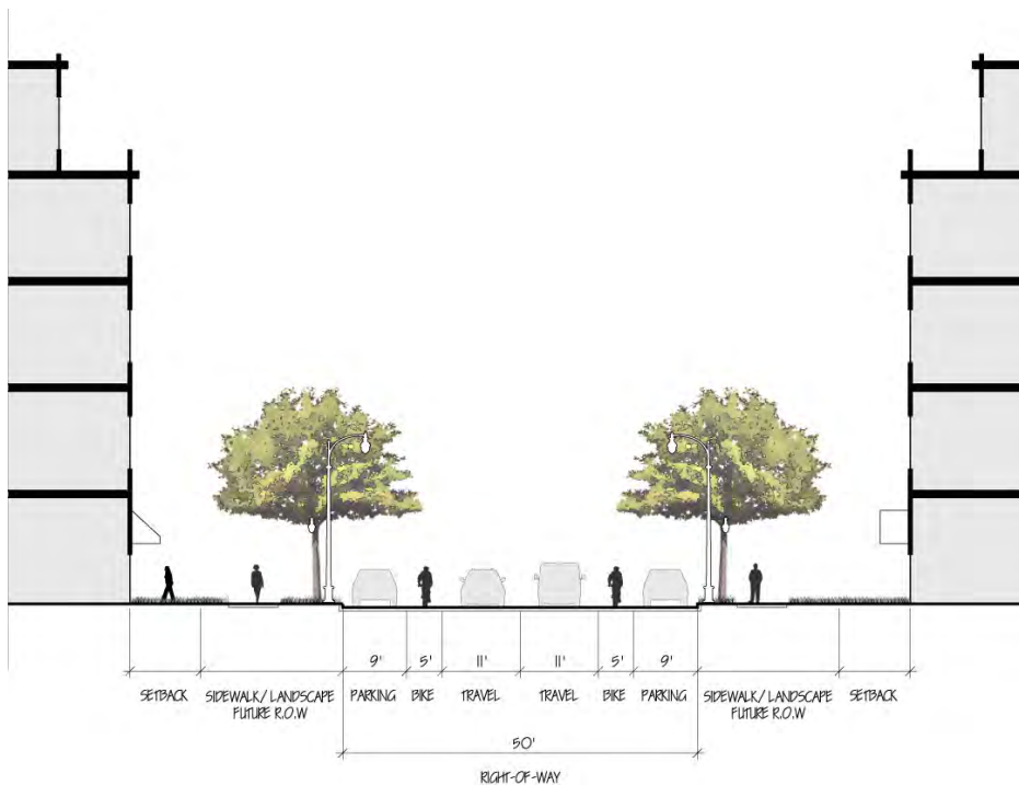
Figure 7-6: Bay Road (East of Bay Road/Tara Road Intersection)
