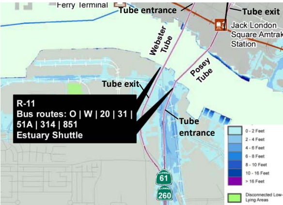
Projected Inundation with 16 inch SLR + 100-yr SWEL
