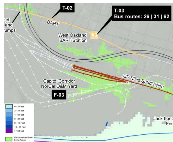
Projected Inundation with 16 inch SLR + 100-yr SWEL
