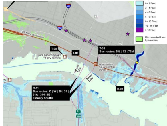
Projected Inundation with 16 inch SLR + 100-yr SWEL
