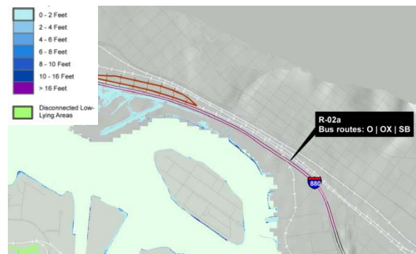
Projected Inundation with 16 inch SLR + 100-yr SWEL
