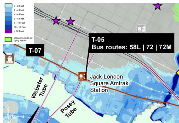
Projected Inundation with 55 inch SLR + 100-yr SWEL
