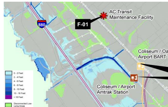
Projected Inundation with 16 inch SLR + 100-yr SWEL
