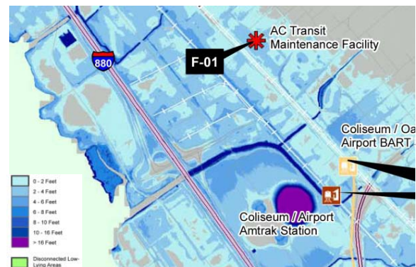
Projected Inundation with 55 inch SLR + 100-yr SWEL
