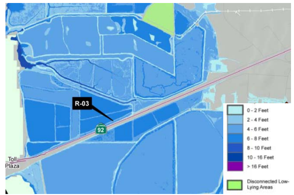
Projected Inundation with 16 inch SLR + 100-yr SWEL
