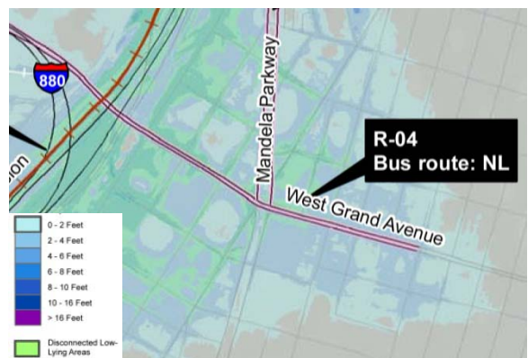
Projected Inundation with 55 inch SLR + 100-yr SWEL
