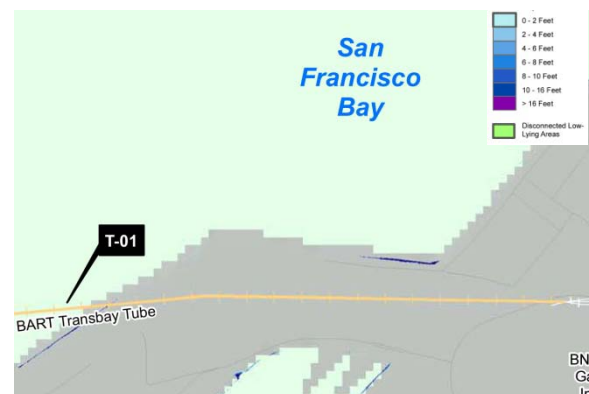
Projected Inundation with 16 inch SLR + 100-yr SWEL
