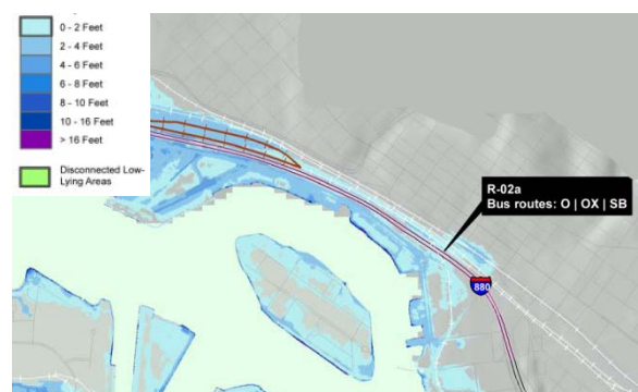
Projected Inundation with 55 inch SLR + 100-yr SWEL
