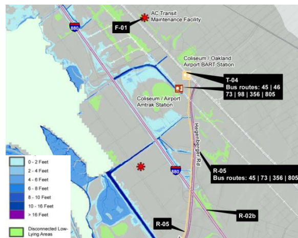
Projected Inundation with 16 inch SLR + 100-yr SWEL
