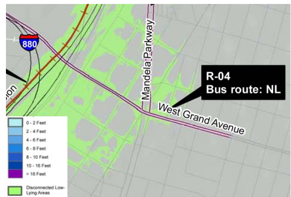
Projected Inundation with 16 inch SLR + 100-yr SWEL
