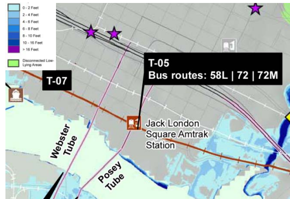
Projected Inundation with 16 inch SLR + 100-yr SWEL
