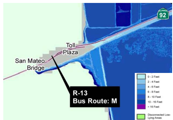
Projected Inundation with 55 inch SLR + 100-yr SWEL
