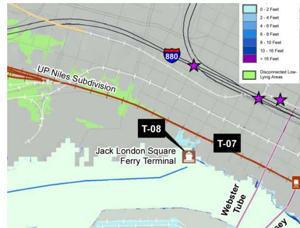
Projected Inundation with 16 inch SLR + 100-yr SWEL
