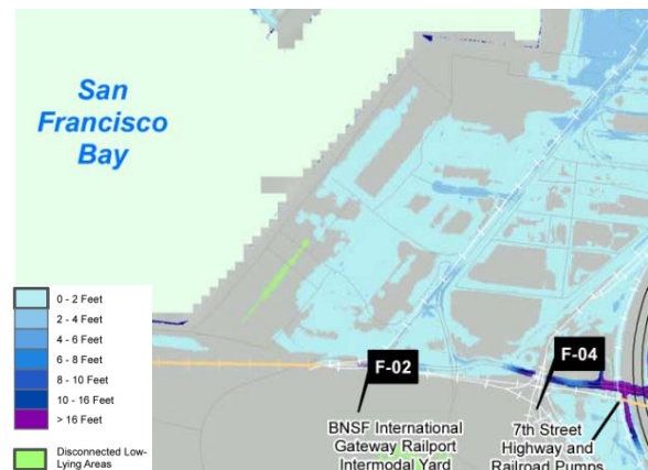
Projected Inundation with 55 inch SLR + 100-yr SWEL
