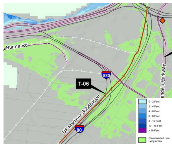
Projected Inundation with 16 inch SLR + 100-yr SWEL
