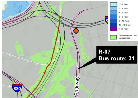
Projected Inundation with 16 inch SLR + 100-yr SWEL
