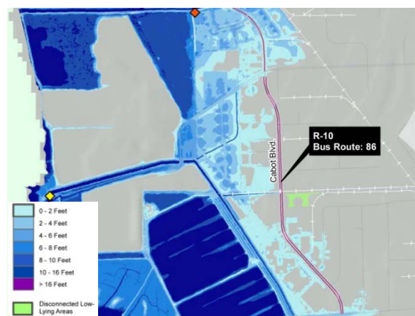
Projected Inundation with 16 inch SLR + 100-yr SWEL
