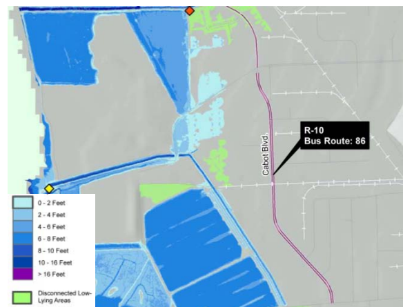
Projected Inundation with 16 inch SLR + 100-yr SWEL
