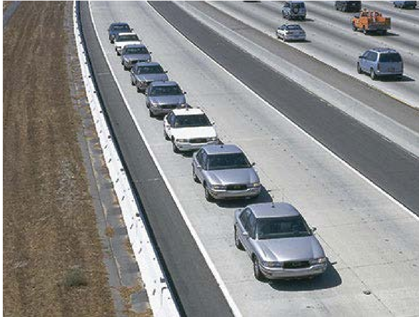
1997 demonstration of the Automated Highway System (AHS) on I-15 in San Diego, CA
