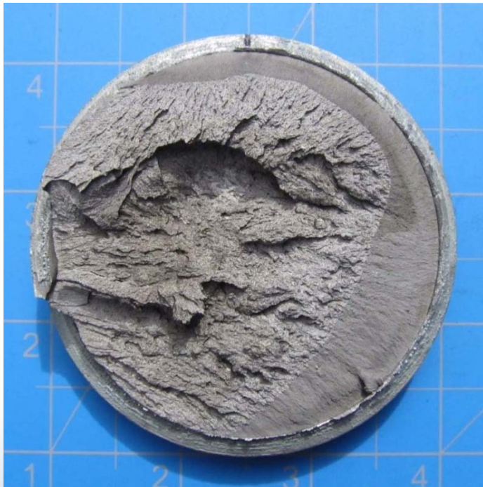
Brittle Failure in Field
